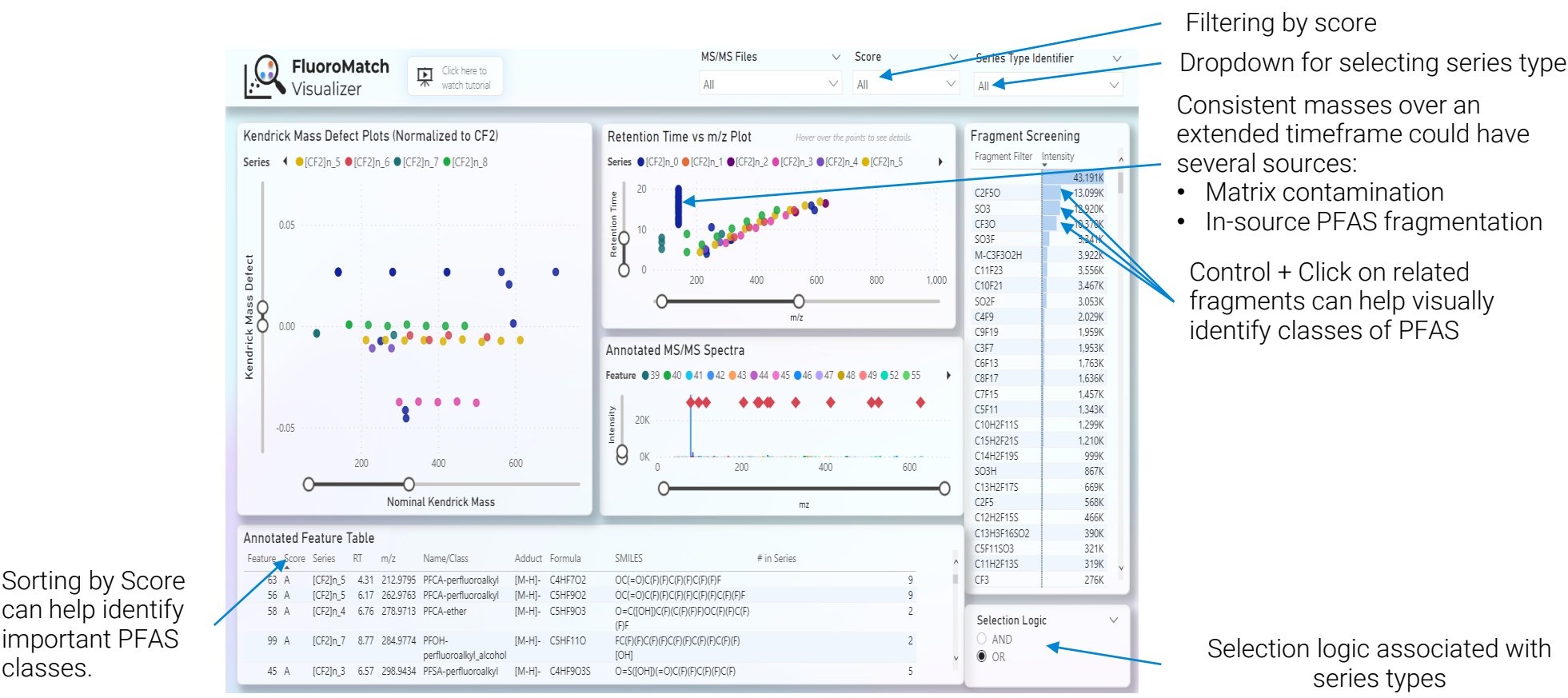
Figure 6: FluoroMatch Visualizer provides interactive mass defect plots, accurate mass vs. retention time plots, MS/MS fragmentation plots, annotation tables, and fragment screening. Selecting and sorting on fragments and features can aid in confirming annotations in homologous series.
