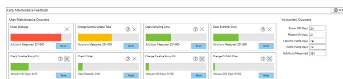
**Figure 3.** To maintain peak ICP-MS performance, EMF prompts maintenance such as cleaning the interface cones, adjusting or replacing the pump tubing, etc. after a specified number of samples have been analyzed.
