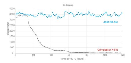
An Agilent J&W DB-5ht column and a competitor's 5ht column were held at 400 °C for 120 hours to evaluate performance and stability. In just 15 hours, the competitor's column drastically lost its performance, measured by plates/meter, despite claiming a 430 °C maximum temperature stability. The J&W DB-5ht column remained stable—even after 40+ hours at the same conditions.
