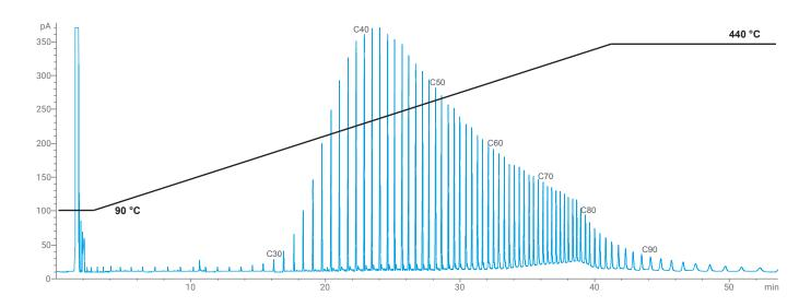
Column: Agilent J&W VF-5ht UltiMetal, 30 m x 0.32 mm x 0.10 µm (p/n CP9096)
