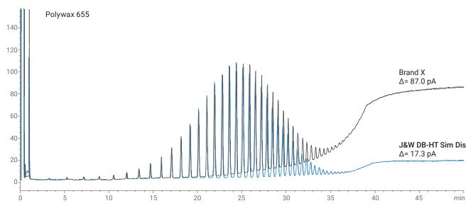
Comparison of Agilent J&W DB-HT Sim Dis and Competitor X Sim Dis columns for polywax 500 analysis. The Agilent column displayed very low bleed and low baseline, even with a 430 °C final temperature.
