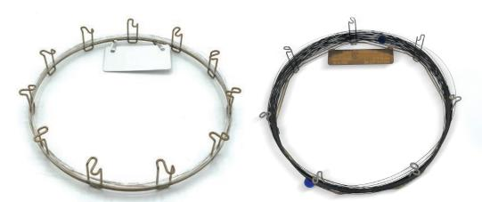
Agilent (column on the right) versus the competition (column on the left). After operating at 400 °C for 25 hours, the competitor's 5ht GC column flaked off, showing signs of depolymerization. The coating on the Agilent J&W DB-5ht GC column remained uniform, and the column maintained its flexibility.
