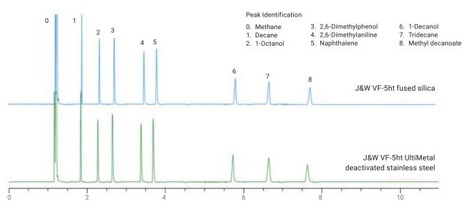
Fused silica and VF-5ht UltiMetal deactivated stainless steel columns after 5 hours at 430 °C.
