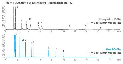
A closer look at the chromatograms after 120 hours at 400 °C. With the competitor's 5ht column, peak tailing is visible for most analytes. Tailing of an alkane, such as *n*-tridecane, proves that the active sites that cause peak tailing are due to stationary phase breakdown. The J&W DB-5ht column shows no sign of phase degradation under the same conditions, proving that the phase is stable after prolonged periods at 400 °C.
