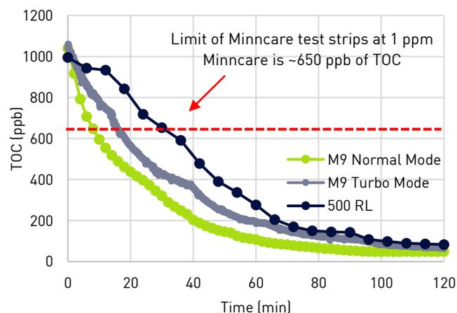
**Figure 1. Simulation of pharmaceutical water system rinse-out following chemical sanitization with Minncare.**
